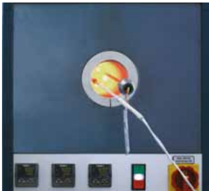
Performance test at 900 °C in a furnace and hydrostatic pressure test
