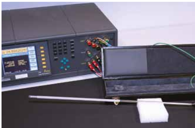
ITS90 calibrated, SPRT (Standard Platinum Resistance Thermometer) reference thermometer
