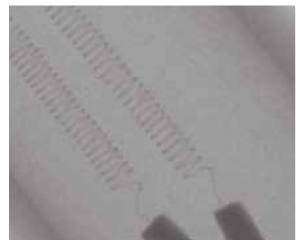
Wire spiral of a wire wound sensor with approx. 20 µm wire diameter
