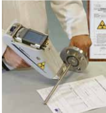
Positive material identification (PMI) and optical quality control
