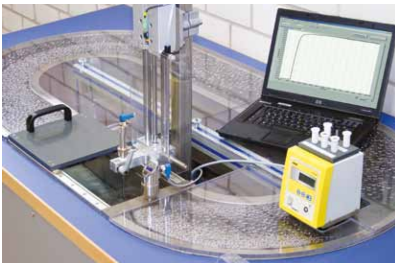
Checking the sensor response time in a water velocity test unit
